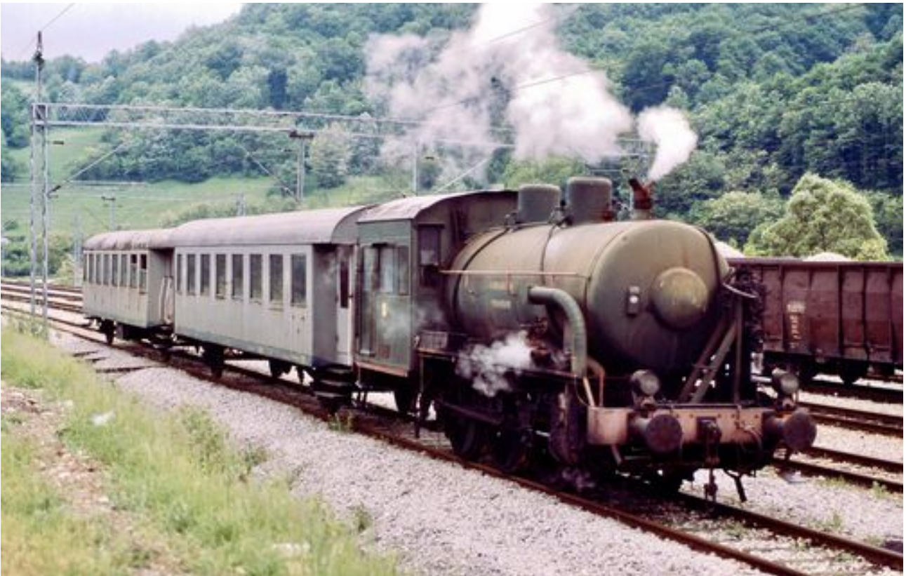
The passenger fireless at Lucani presumably seen at the electrified mainline junction at Dragacevo. It's based on a Yugoslavian-built USA tank (class 62) © Roland Beier
