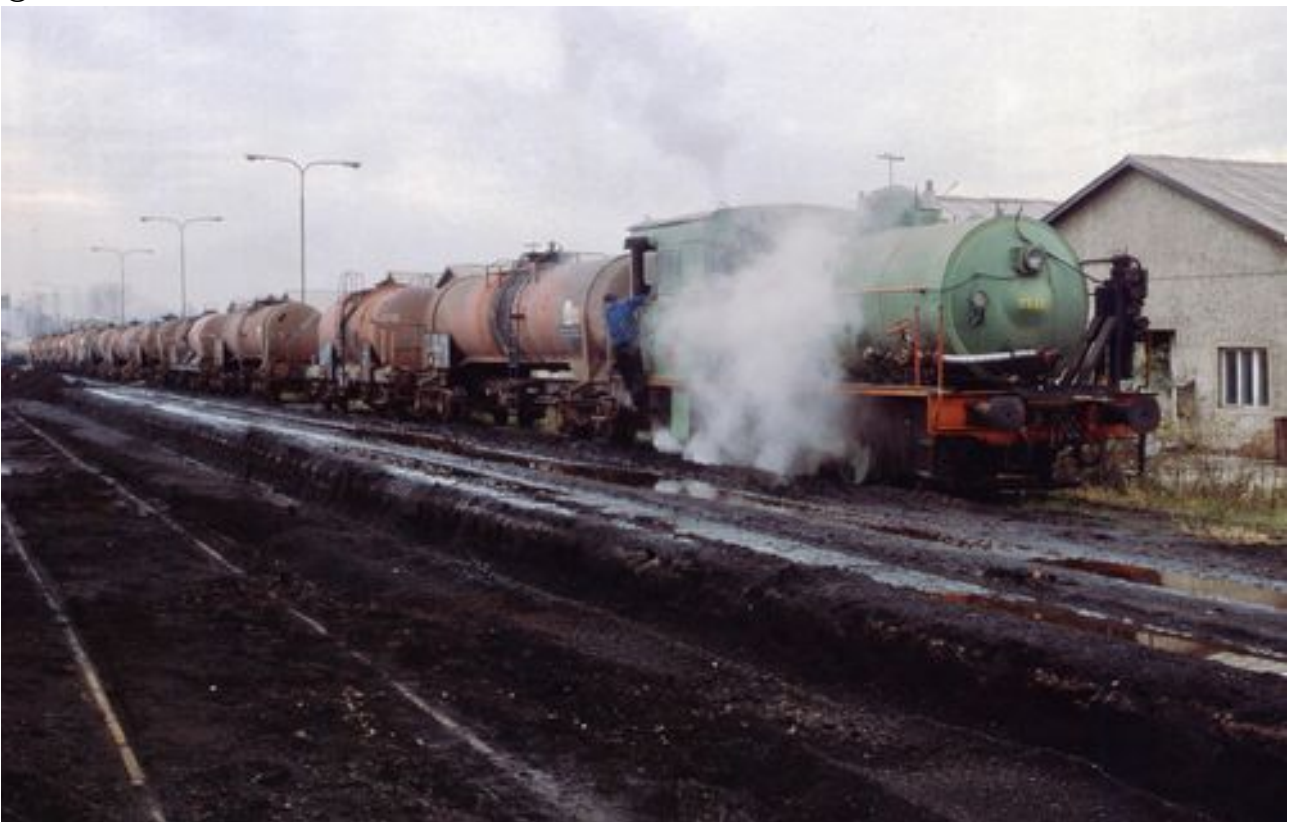
The passenger fireless at Lucani presumably seen at the electrified mainline junction at Dragacevo. It's based on a Yugoslavian-built USA tank (class 62) © Roland Beier
